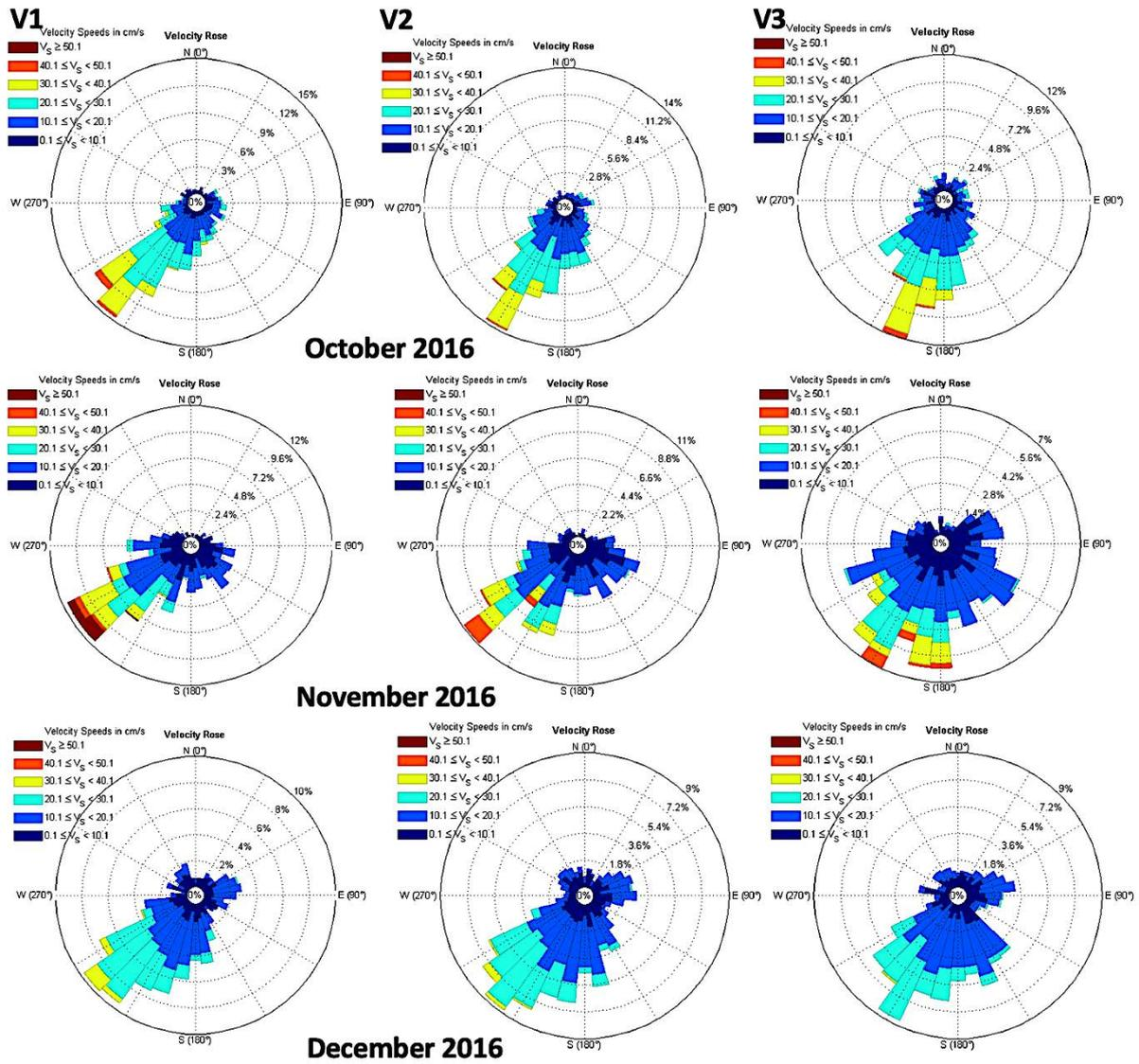
Figure 8: Monthly current intensity and direction collected offshore Dakhla at INRH METOCEAN buoy at depths 10m (V1), 20m (V2) and 30m (V3) during autumn 2016.
